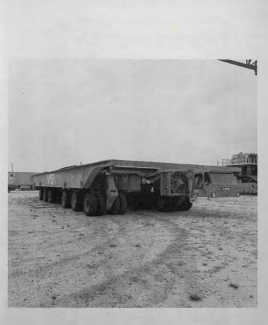
Figure 16. Payload Canister Transporter.
